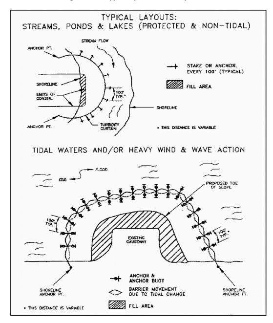
Figure 2. Two typical layouts of a turbidity curtain.
