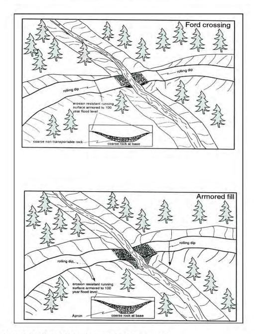
Figure X-15. Typical ford and armored fill stream crossings.
