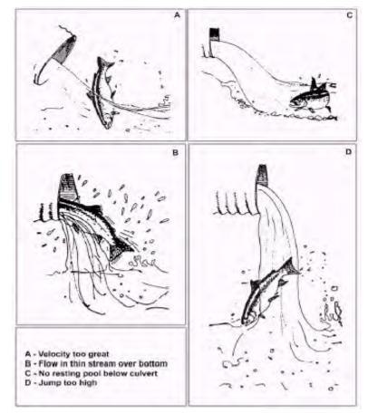
**Figure 4.2 Fish passage barrier conditions at culverted stream crossings.** (*California Salmonid Stream Habitat Restoration Manual; Chapter IX, California Dept. of Fish and Wildlife, Flosi et. al 2002.*)
