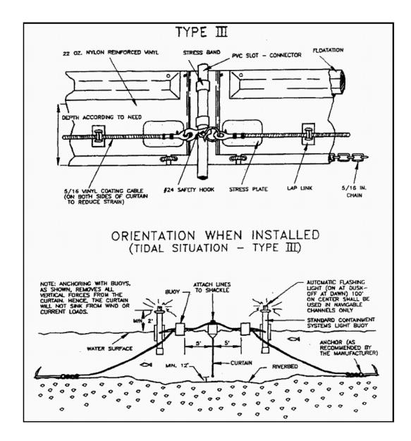
Figure 1. Turbidity Curtain - Type III, including tidal situation.
