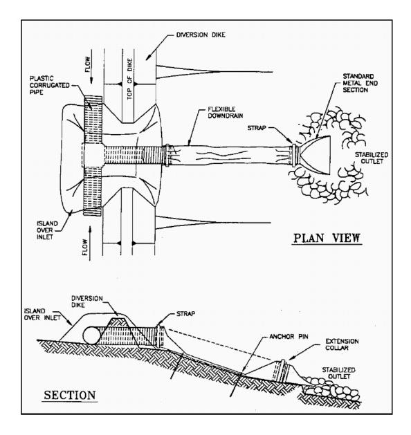
Source: McCullah, J. 1992. Erosion and Sediment Control Standards Design Manual <u>– County of Shasta</u>. Prepared for the Western Shasta RCD. Redding CA. 187 p.
