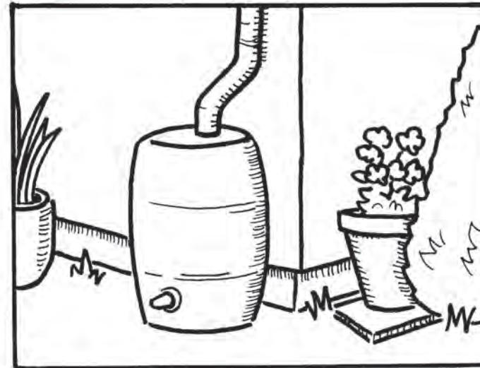
MAINTENANCE: Rain barrels require regular draining after rainstorms and removal of leaves and debris collected on screens. Always check that the overflow is clear and directed to an appropriate location. Fine mesh screens should be used to seal lids and vents. A hole larger than 1/16 of an inch can allow mosquito access and result in significant larvae production.
