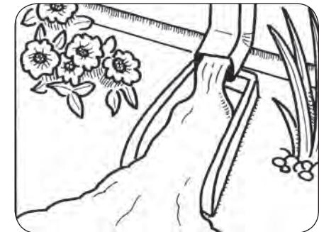
**A HOSE ADAPTER** is a neat option (Drought Buster East Connect is pictured) that allows a standard garden hose to connect directly to a downspout. The hose can be moved to different locations of your yard when it rains, allowing the water to SPREAD out through the landscape. It is perfect for watering trees or keeping any one area from becoming too saturated.
