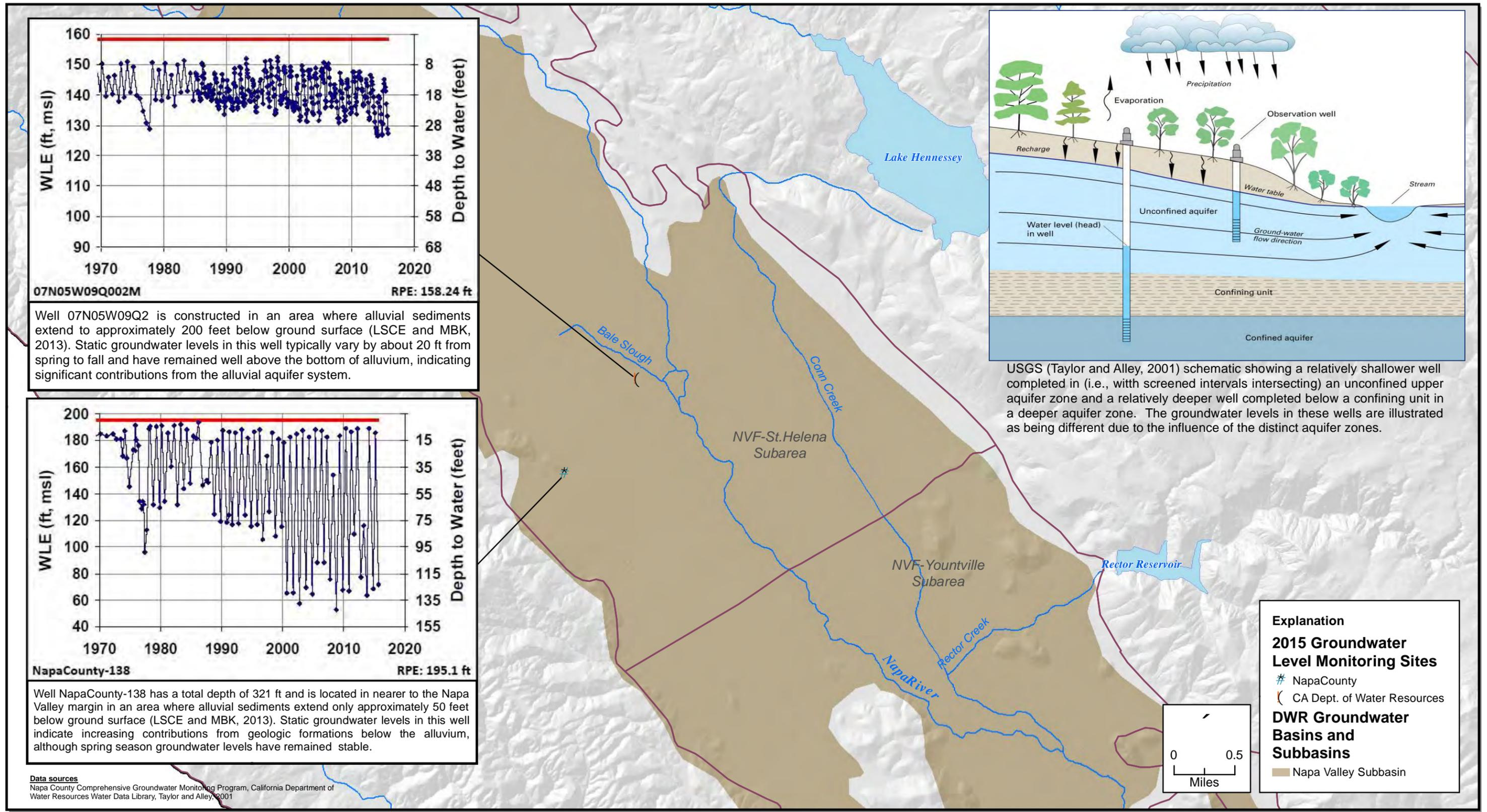
Well 07N05W09Q2 is constructed in an area where alluvial sediments extend to approximately 200 feet below ground surface (LSCE and MBK, 2013). Static groundwater levels in this well typically vary by about 20 ft from spring to fall and have remained well above the bottom of alluvium, indicating significant contributions from the alluvial aquifer system.
