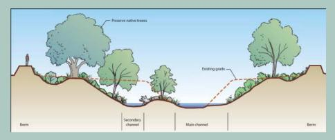
Instead of cutting continuous floodplain benches we have created a series of expansion areas separated by narrower sub-reaches. The expansions and contractions break up the existing long glides and force riffle-pool formation. Pools create summer thermal refugia while riffles create spawning habitat. Expansion areas also provide high velocity refugia for juvenile fish and a location for fine sediment to settle out.
