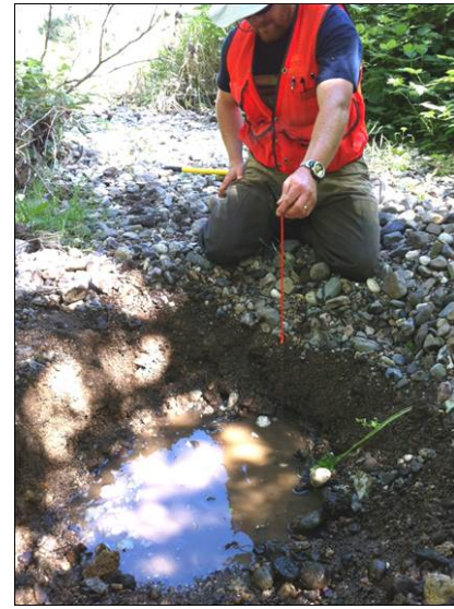
Recovering a buried scour chain from the river.
