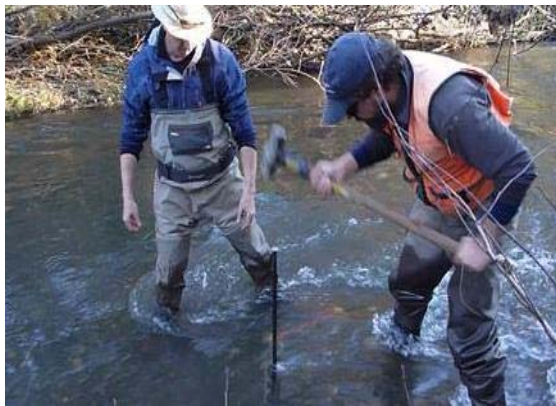
Installing a scour chain.
