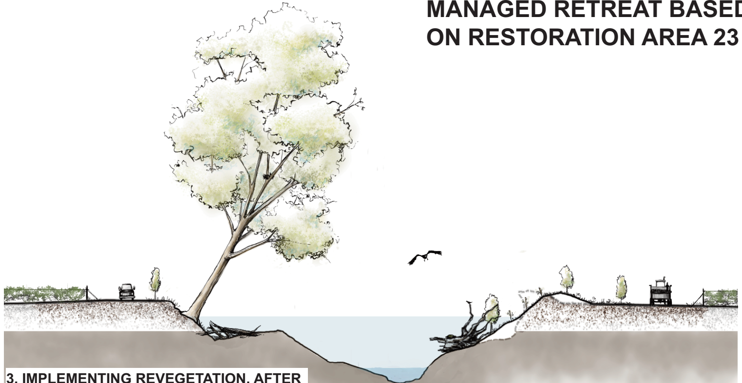
3. IMPLEMENTING REVEGETATION. AFTER BANK ERODES IT IS SHAPED TO A 2 OR 3:1 SLOPE. WILLOWS ARE SPRIGGED INTO THE BASE OF THE BANK AND OTHER NATIVE TREES ARE PLANTED
