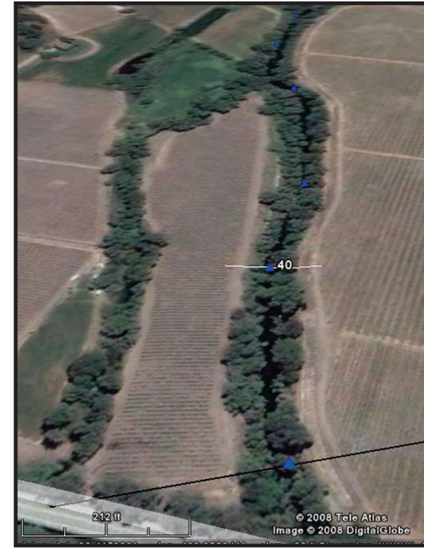
w:d = 3.8. These reaches tend to be dominated by continuous pools with little shelter for fish, have high rates of redd scour and erosion/slumping on both banks, and to have aging riparian trees that are not regenerating
