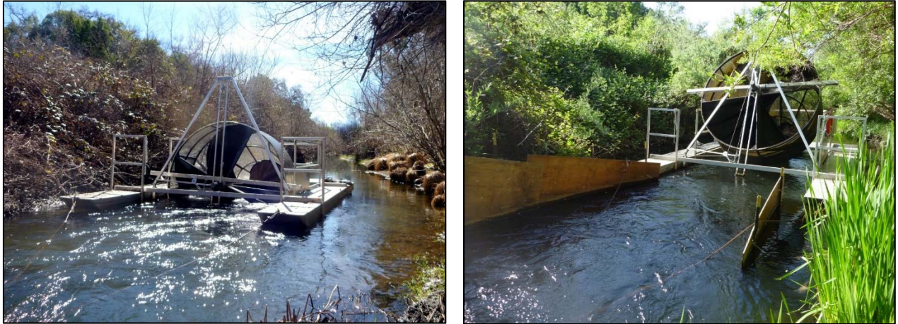
Figure 7. Left: rotary screw trap in operation in February, Right: rotary screw trap tilted out of water due to low flow in late April (both photos taken facing downstream)
