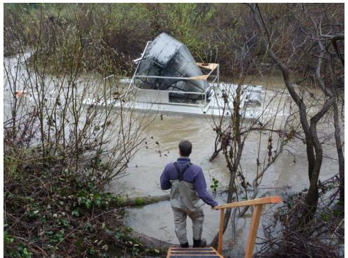
Rotary screw trap with cone tilted during high flows (1,200 cfs)
