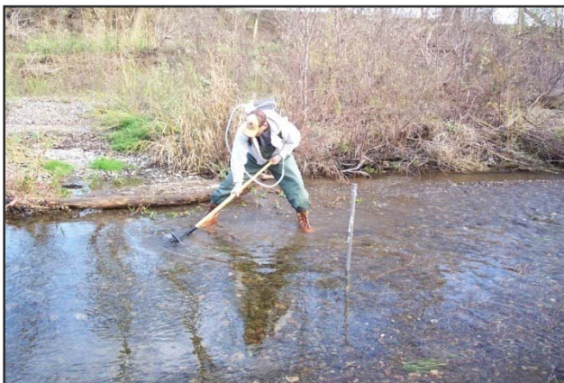
Spawning gravel is manually cleaned to a depth of ~ 0.95 feet prior to driving in the standpipe to simulate the cleaning effect of redd construction.
