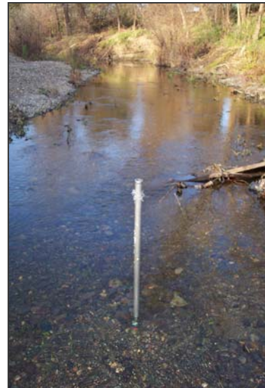
Standpipe driven into the bed of the Napa River
