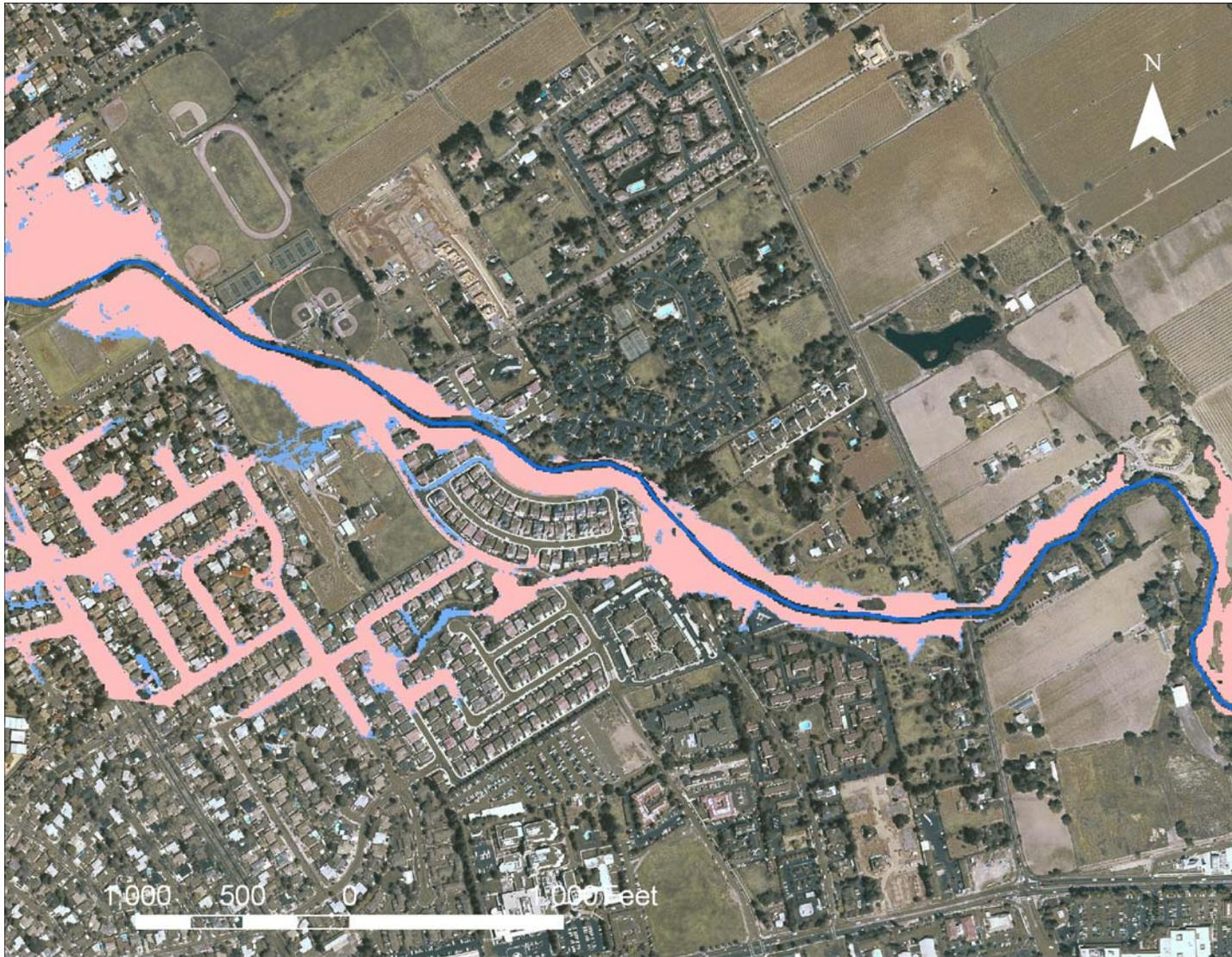
Figure 21b. Downstream view of maximum extent of inundation for Scenario 4 (pink) compared with the baseline inundation extent (light blue) for the 100-yr flood event, areas where light blue is visible indicate reduction in inundation extent under scenario 4
