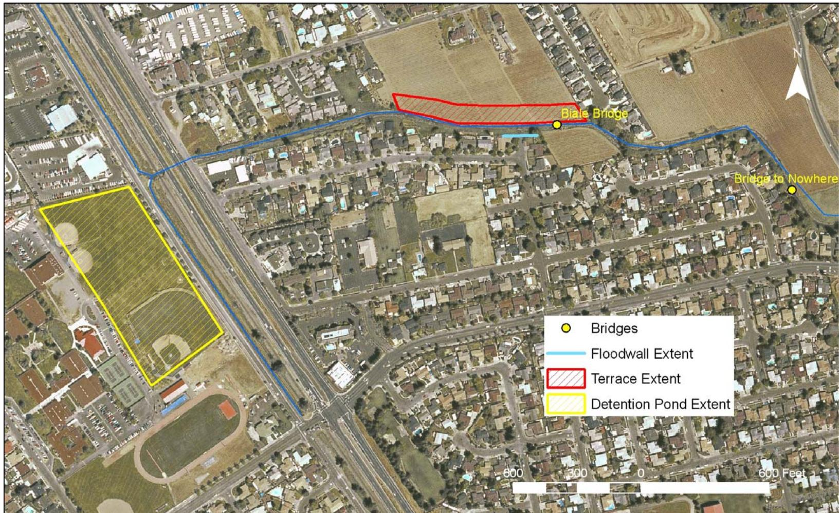
Figure 4. Scenario elements including bridges that were removed, the extent of the floodwall near Lassen Street, the extent of the terrace, and the location and extent of the detention pond west of the highway
