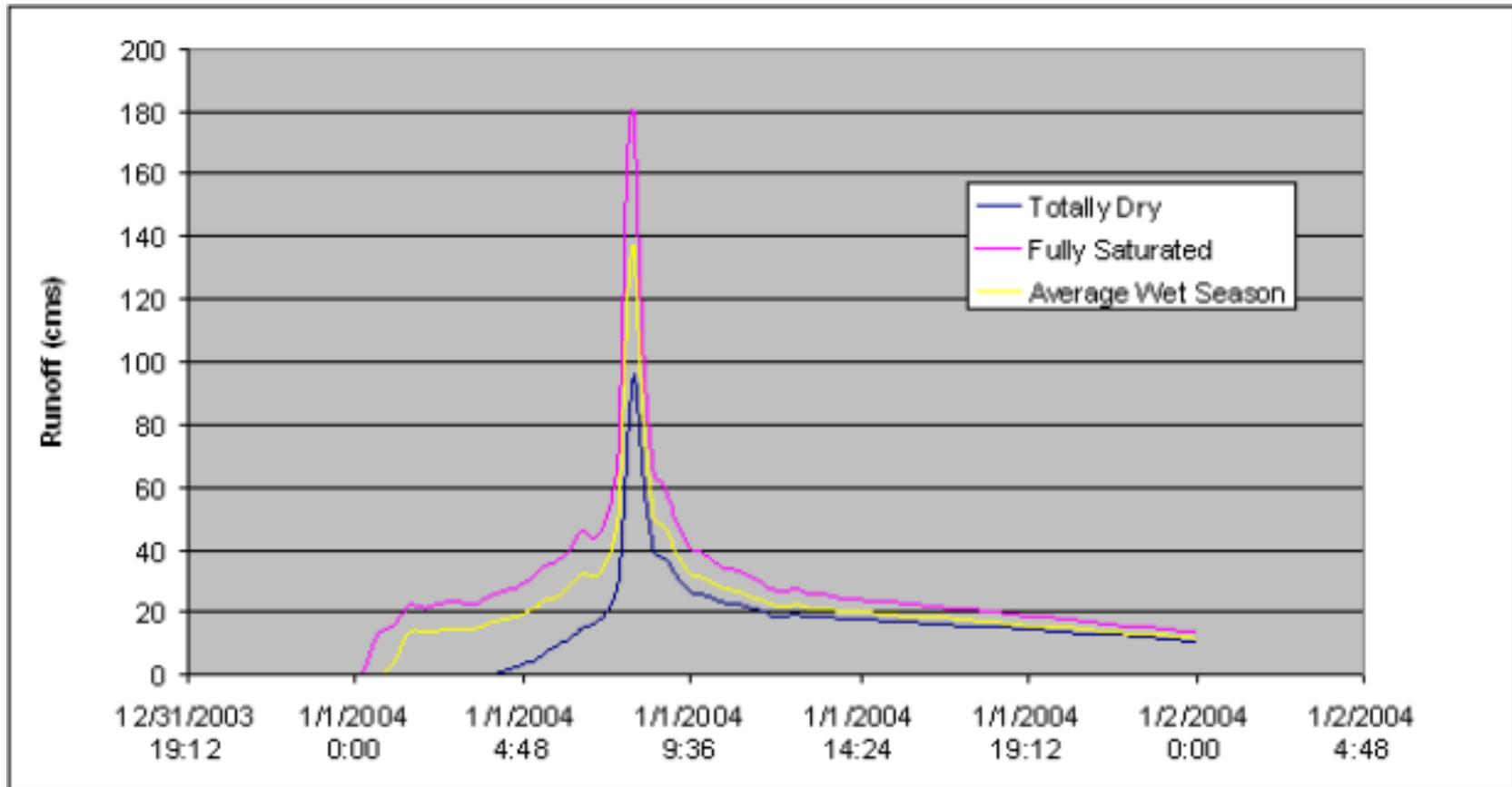
Figure 1. Effect of Initial Conditions on Runoff in MIKE 11
