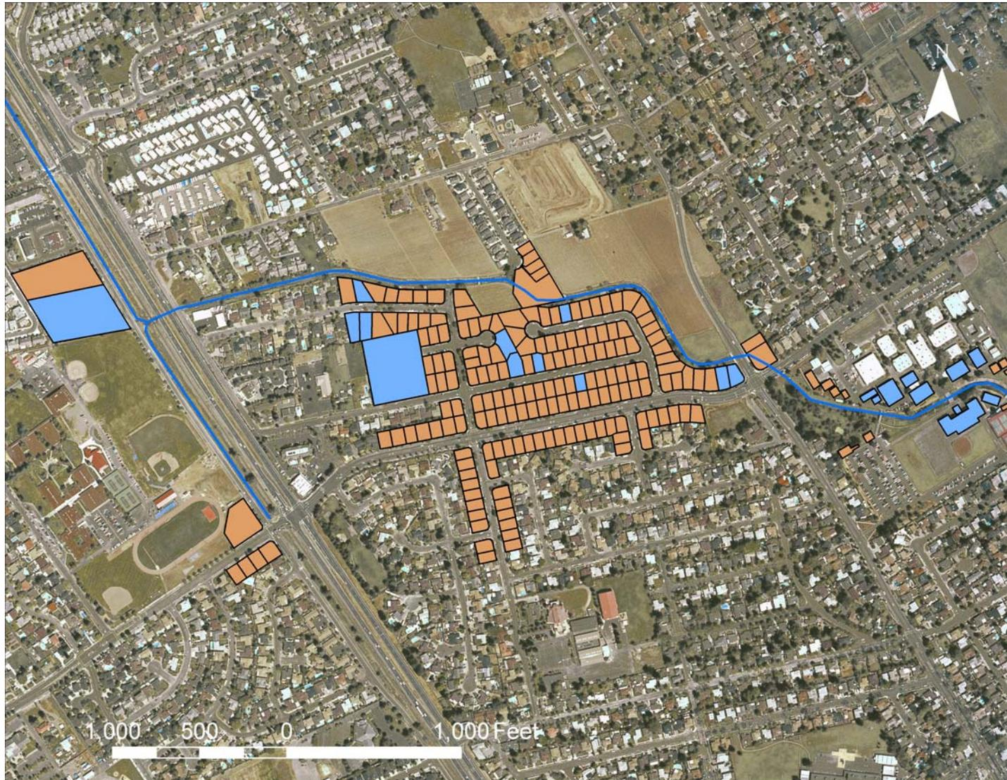
Figure 9a. Comparison of the maximum inundation depths for the 100-yr flood event for the baseline condition with the surveyed finished floor elevations, inundated parcels are shown in blue (upstream view)
