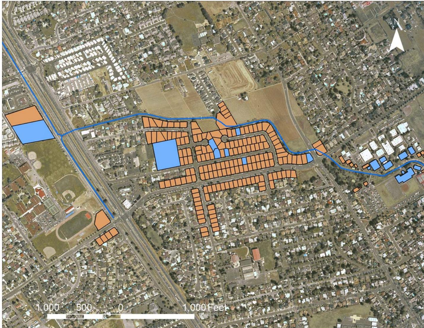
Figure 18. Comparison of the maximum inundation depths for the 100-yr flood event for Scenario 3 with the surveyed finished floor elevations, inundated parcels are shown in blue
