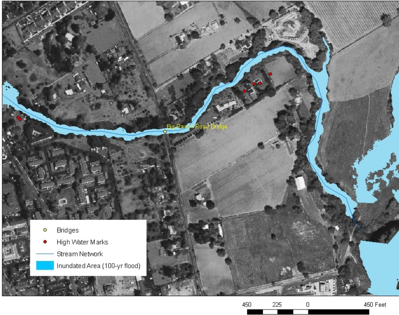
Figure 14. Effect of Flood Terraces on 100-year Water Level
