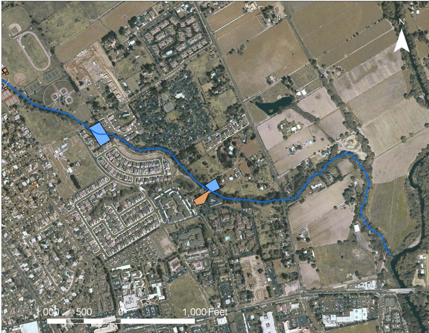
Figure 9b. Comparison of the maximum inundation depths for the 100-yr flood event for the baseline condition with the surveyed finished floor elevations, inundated parcels are shown in blue (downstream view)
