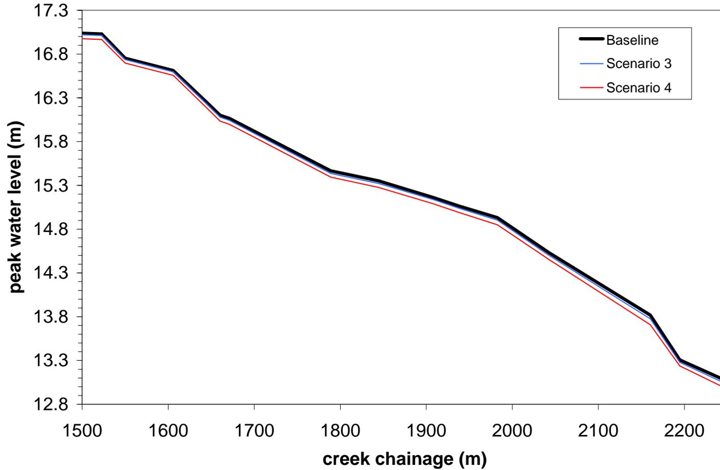
Figure 17c. Peak water levels during the 100-yr flood event for the baseline condition and for Scenarios 3-4 (chainage 1500 – 2250 m)
