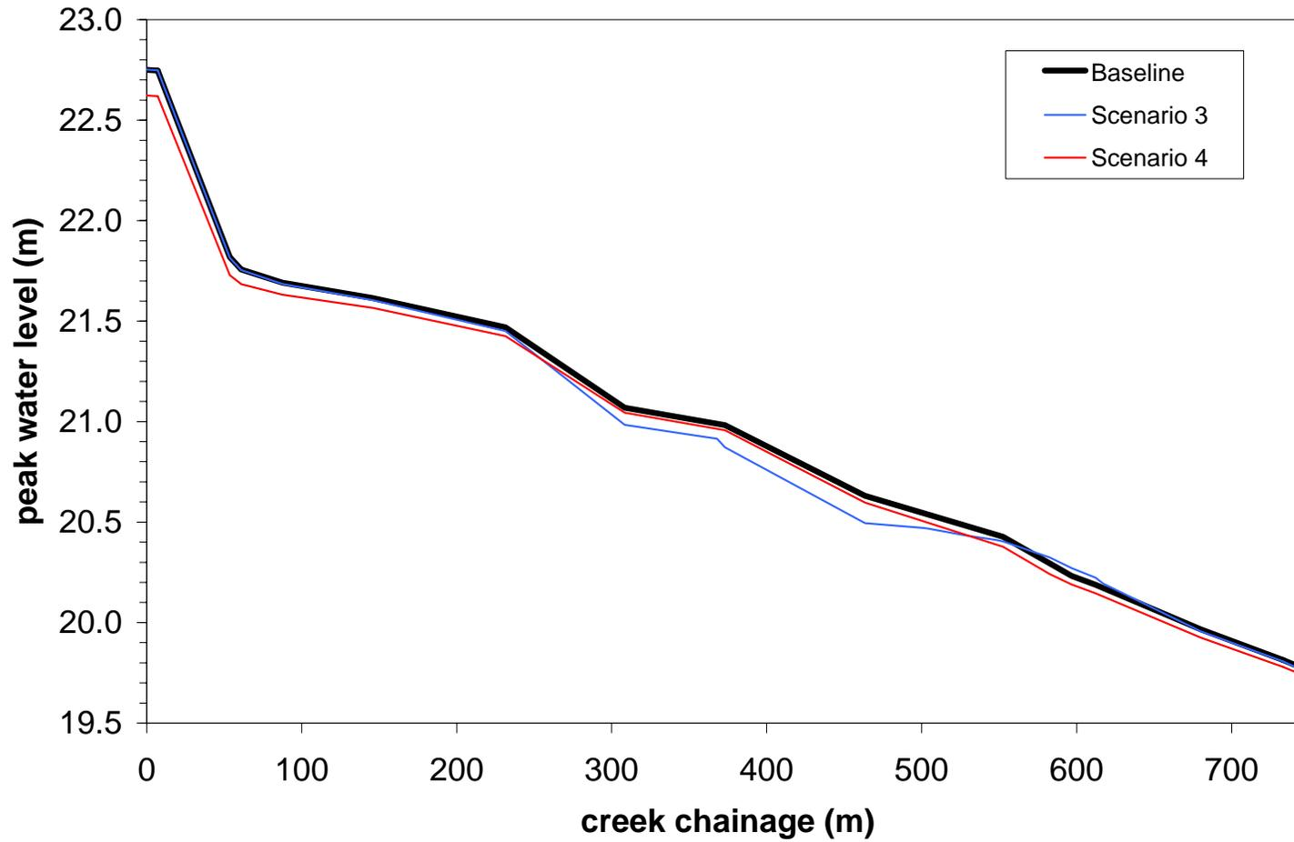
Figure 17a. Peak water levels during the 100-yr flood event for the baseline condition and for Scenarios 3-4 (chainage 0 – 750 m)
