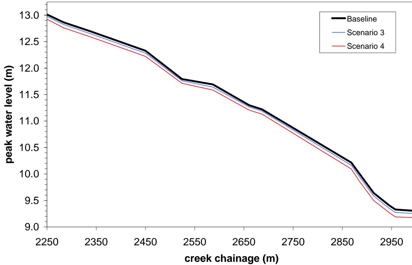
Figure 17d. Peak water levels during the 100-yr flood event for the baseline condition and for Scenarios 3-4 (chainage 2250 – 3000 m)
