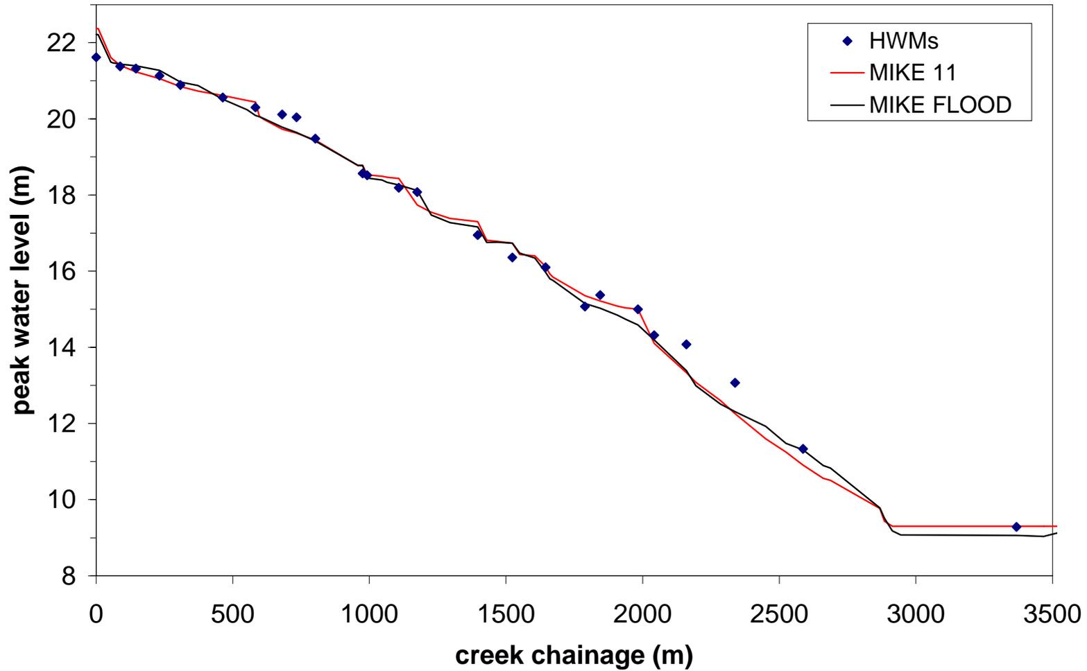
Figure 3. Peak water level comparison between measured high water marks (HWMs), stand-alone MIKE 11 simulated water levels and MIKE FLOOD simulated water levels
