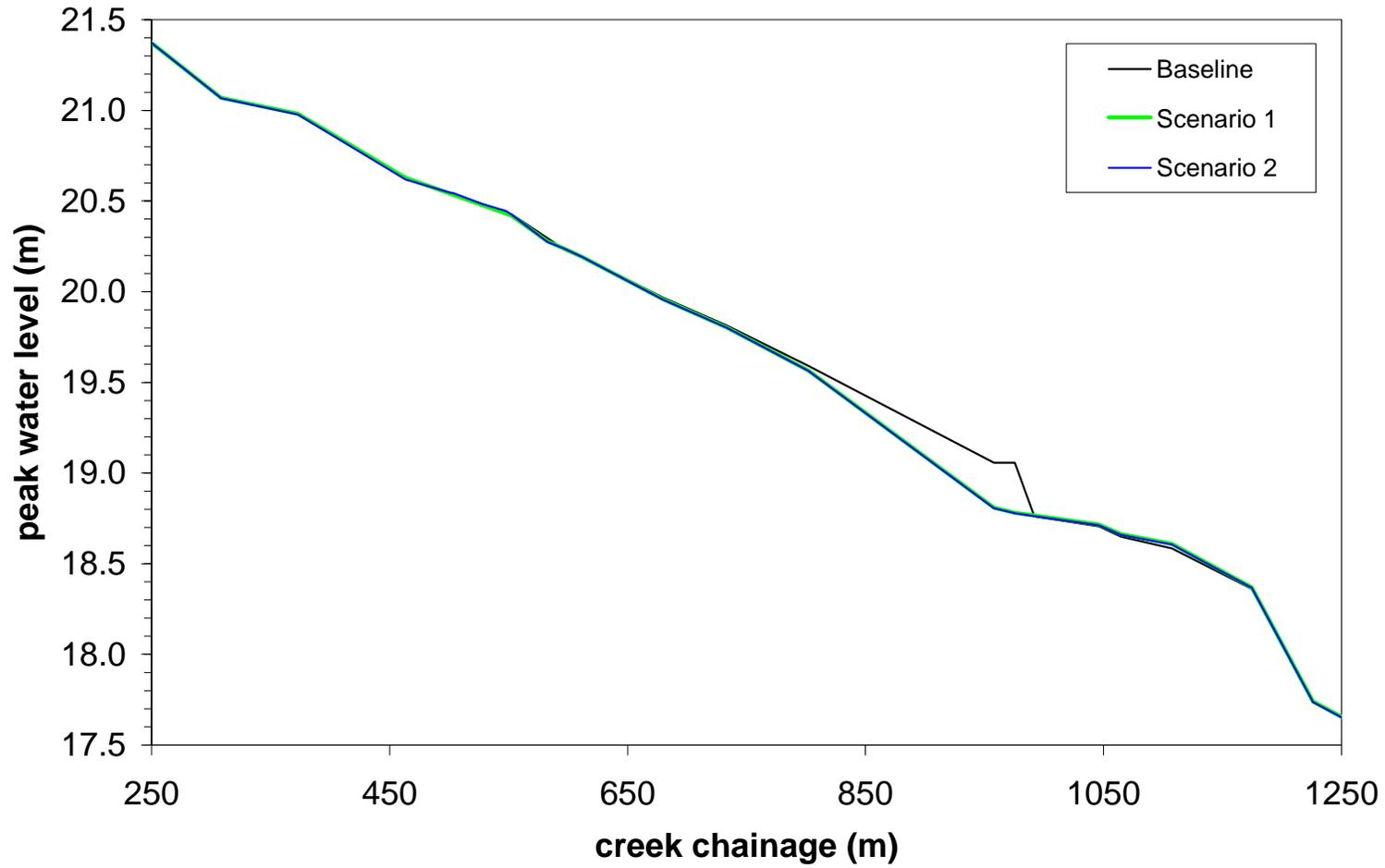
Figure 12. Peak water levels during the 100-yr flood event for the baseline condition and for Scenarios 1-2 in the vicinity of the removed bridges
