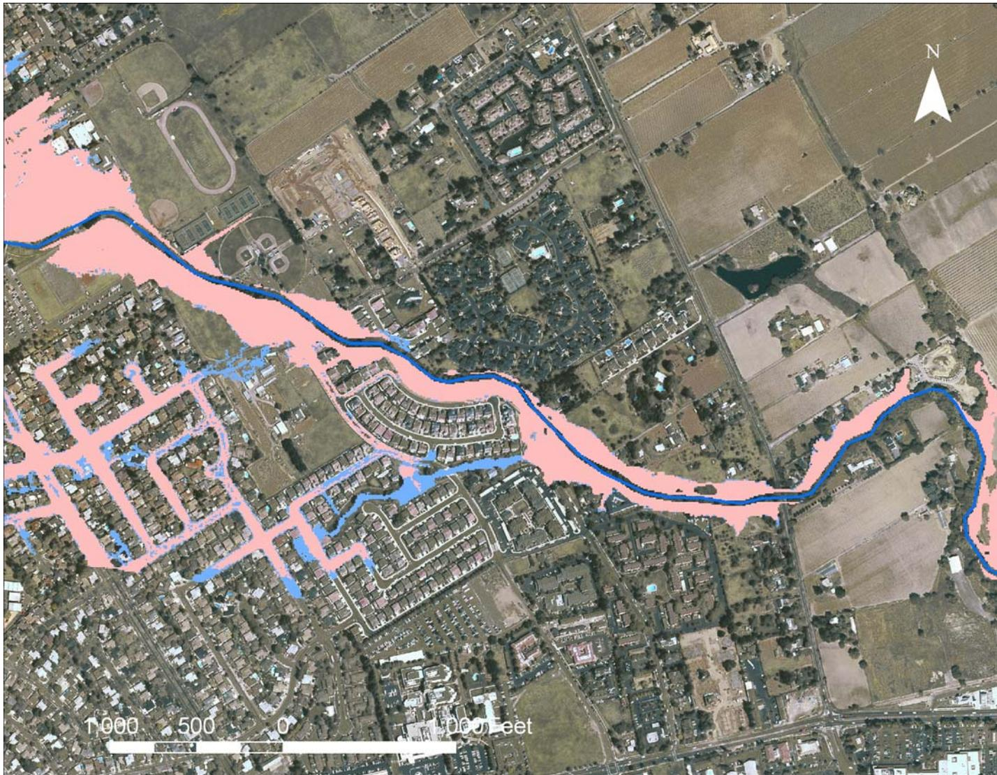
Figure 16b. Downstream view of maximum extent of inundation for Scenario 3 (pink) compared with the baseline inundation extent (light blue) for the 100-yr flood event, areas where light blue is visible indicate reduction in inundation extent under scenario 3
