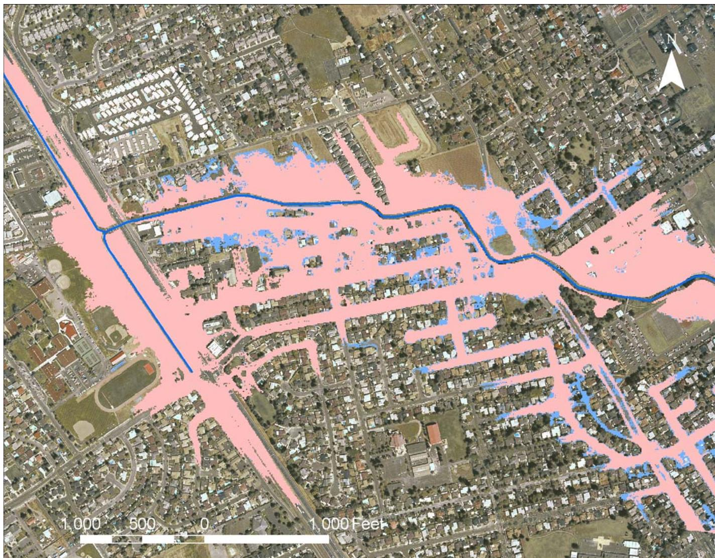
Figure 16a. Upstream view of maximum extent of inundation for Scenario 3 (pink) compared with the baseline inundation extent (light blue) for the 100-yr flood event, areas where light blue is visible indicate reduction in inundation extent under scenario 3
