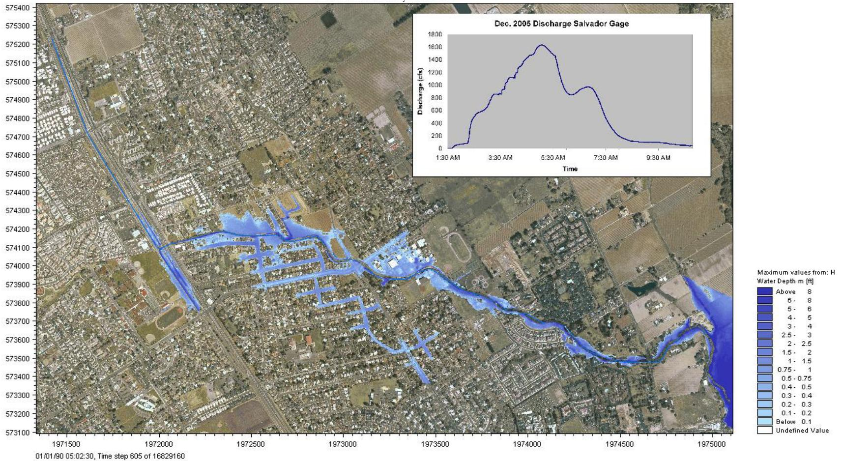
Figure 5. Maximum inundation depths (m) and hydrograph at the Big Ranch Road gage for the December 31, 2005 flood event
