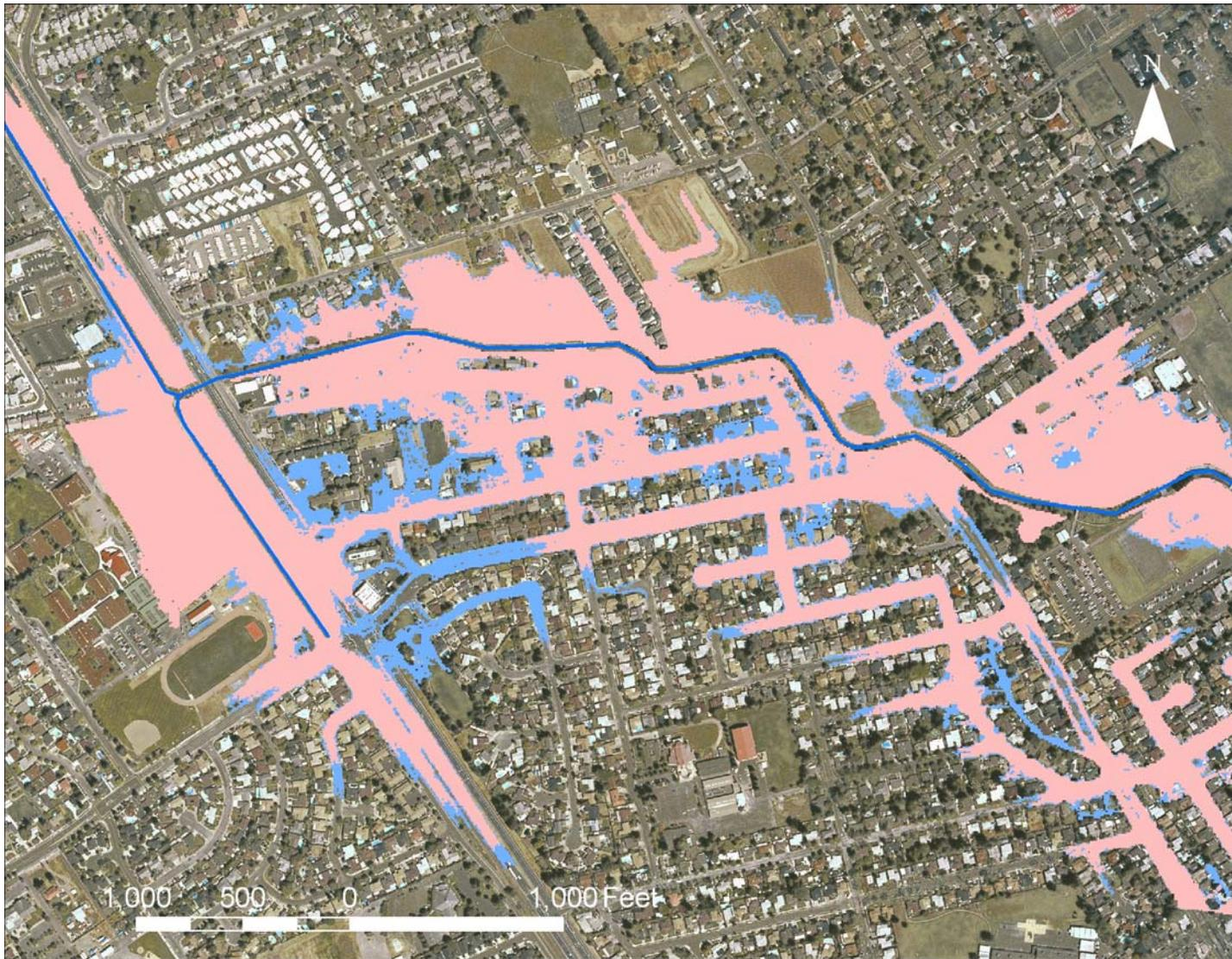
Figure 21a. Upstream view of maximum extent of inundation for Scenario 4 (pink) compared with the baseline inundation extent (light blue) for the 100-yr flood event, areas where light blue is visible indicate reduction in inundation extent under scenario 4
