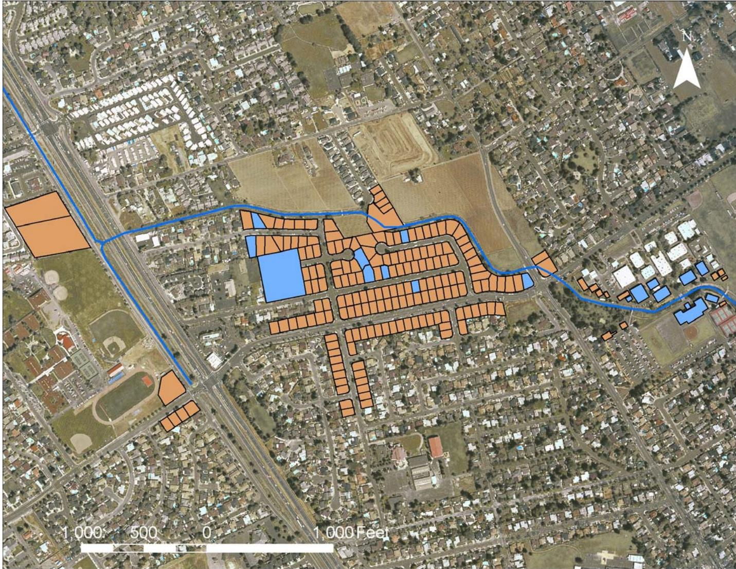
Figure 22. Comparison of the maximum inundation depths for the 100-yr flood event for Scenario 4 with the surveyed finished floor elevations, inundated parcels are shown in blue
