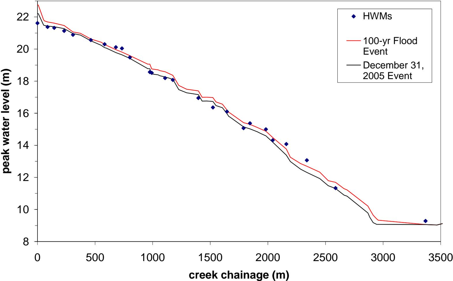
Figure 8. Peak water levels during the 100-yr flood event and comparison with peak water levels during the December 31, 2005 event
