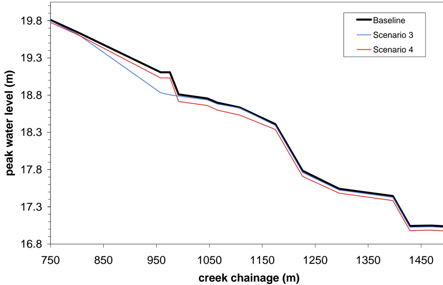
Figure 17b. Peak water levels during the 100-yr flood event for the baseline condition and for Scenarios 3-4 (chainage 750 – 1500 m)
