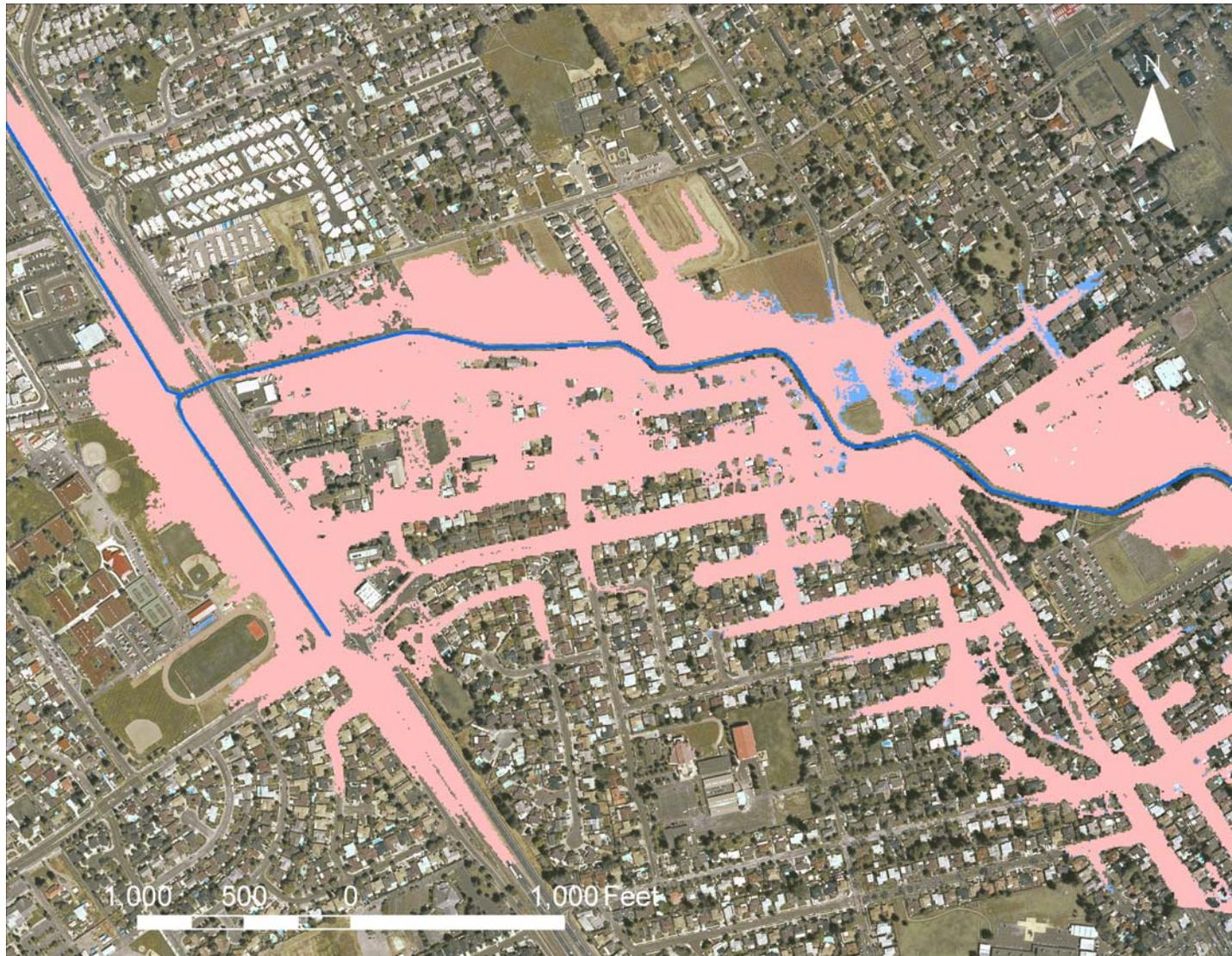
Figure 11. Maximum extent of inundation for Scenario 1 (pink) compared with the baseline inundation extent (light blue) for the 100-yr flood event, areas where light blue is visible indicate reduction in inundation extent under scenario 1
