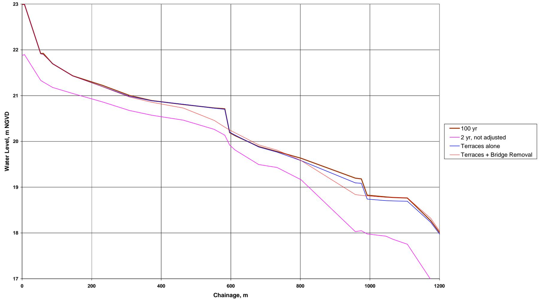
Figure 15. Effect of Highway Bridge Improvement on 100-year Water Level
