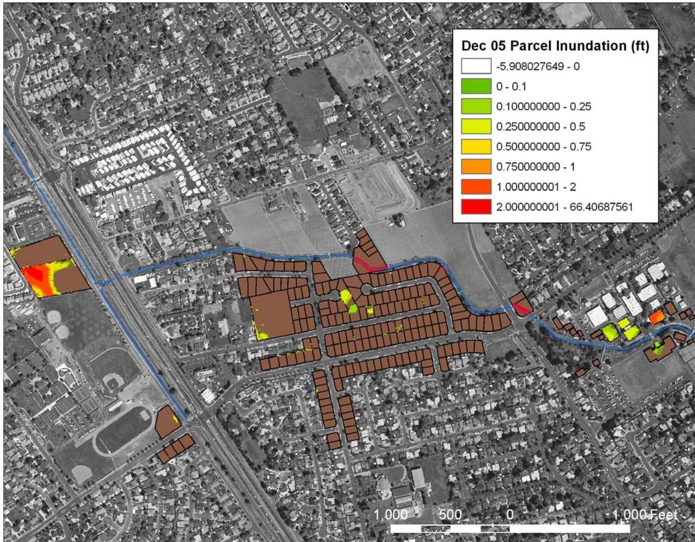
Figure 6a. Comparison of the maximum inundation depths for the December 31, 2005 flood event with the surveyed finished floor elevations showing parcel inundation depths in feet (upstream view)
