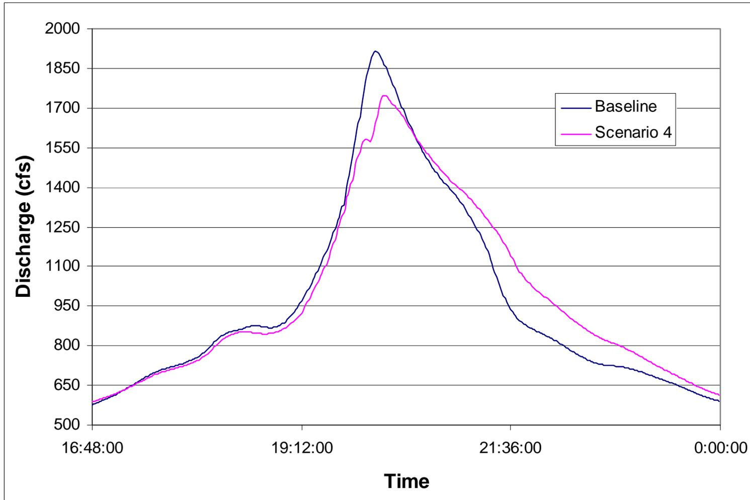
Figure 19. Comparison of the baseline and Scenario 4 hydrographs along Salvador Creek just downstream of the highway crossing
