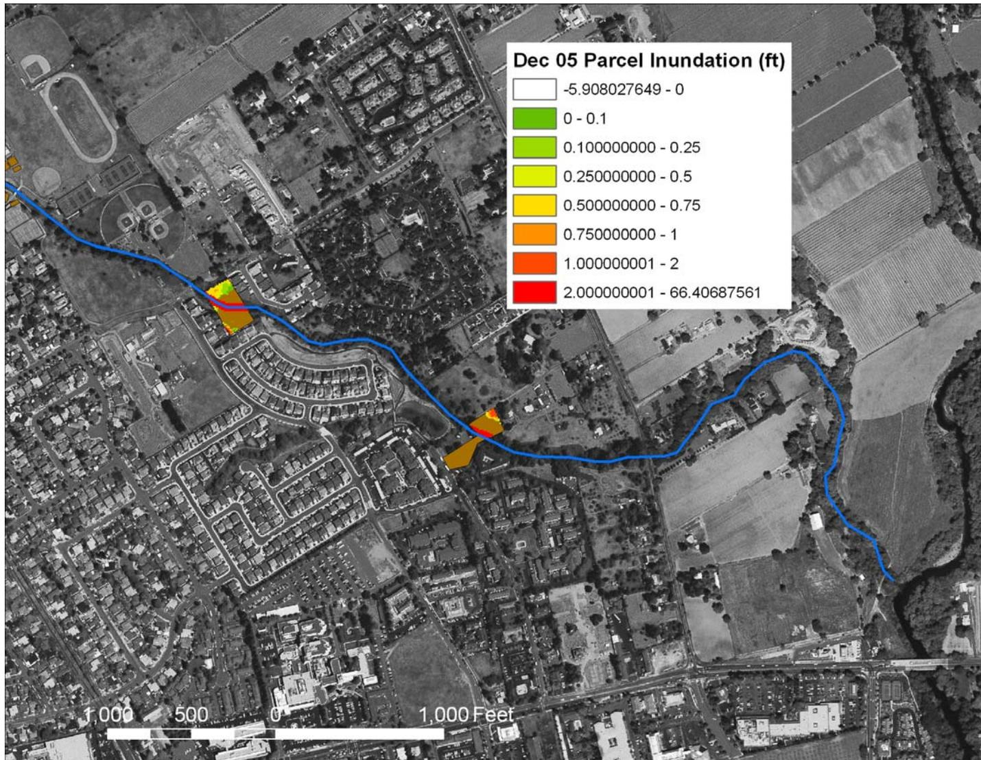
Figure 6b. Comparison of the maximum inundation depths for the December 31, 2005 flood event with the surveyed finished floor elevations showing parcel inundation depths in feet (downstream view)
