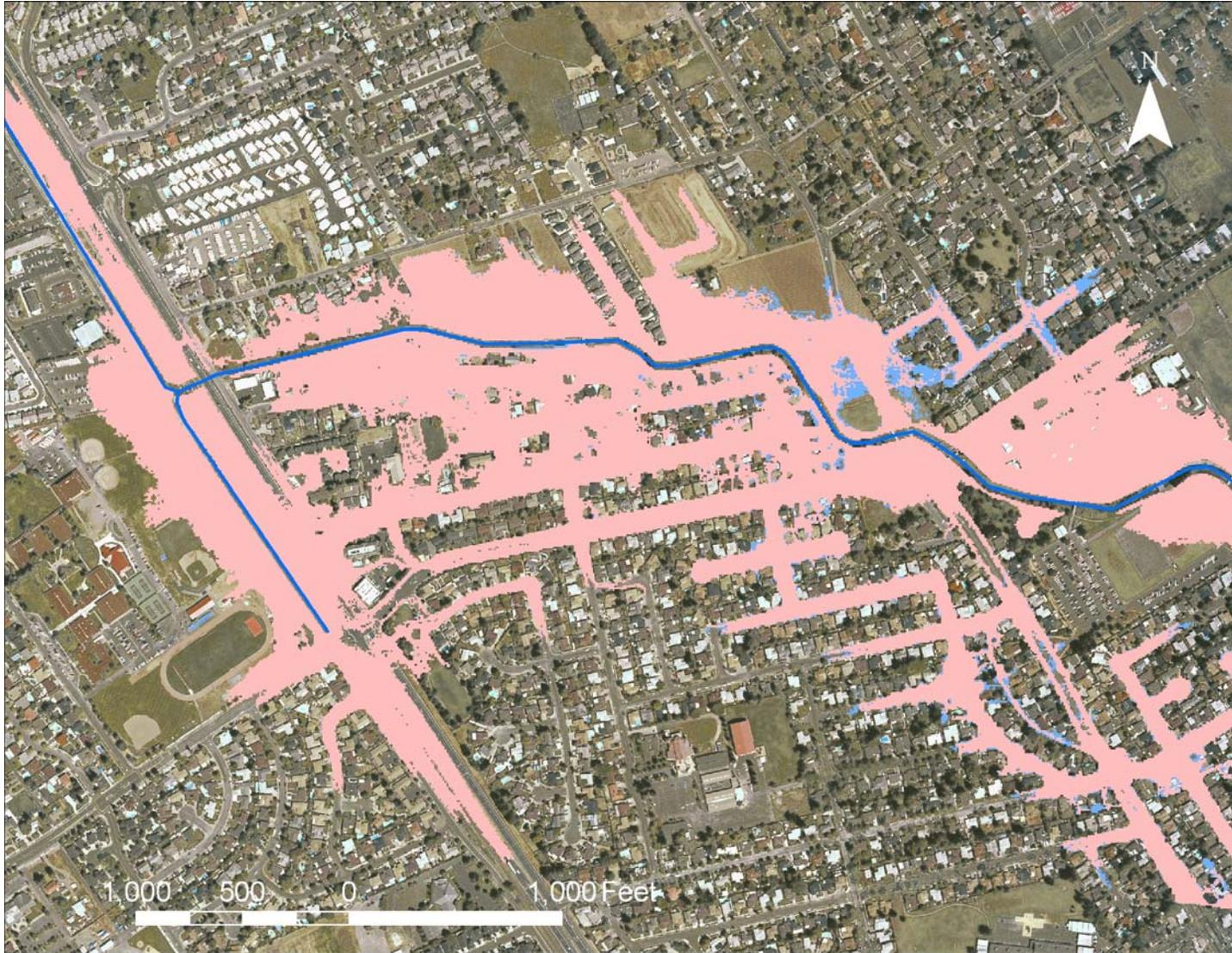
Figure 14. Maximum extent of inundation for Scenario 2 (pink) compared with the baseline inundation extent (light blue) for the 100-yr flood event, areas where light blue is visible indicate reduction in inundation extent under scenario 2
