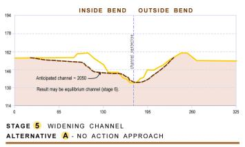
Figure 13. Typical existing conditions and conceptual design for Reach 3
