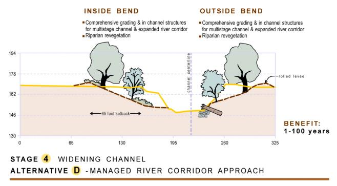
Figure 11. Typical existing conditions and conceptual design for Reach 1
