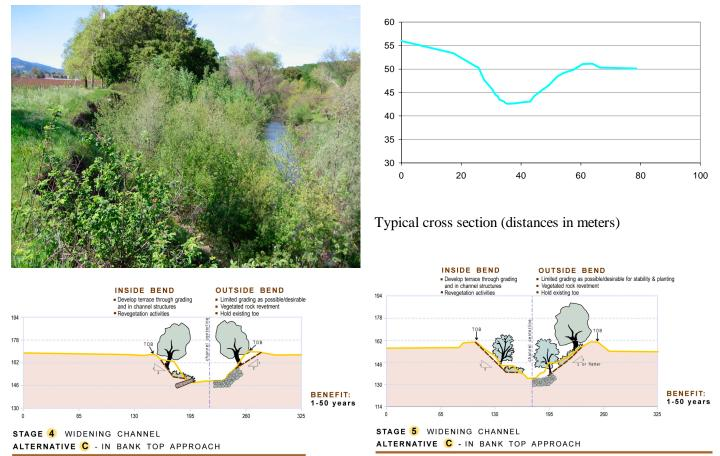
Figure 12. Typical existing conditions and conceptual design for Reach 2
