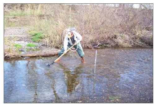
Spawning gravel is manually cleaned to a depth of 0.95 feet prior to driving in the standpipe to simulate the cleaning effect of redd construction.
