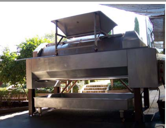
The L eq for a destemmer at 70 feet is 66.7 dBA.
