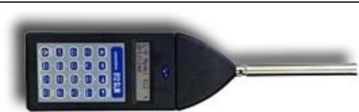
Short-term monitoring was conducted at 20 locations throughout the County using a Larson-Davis Model 812 Precision Type 1 sound level meter placed 5 feet above the ground on a tripod.
