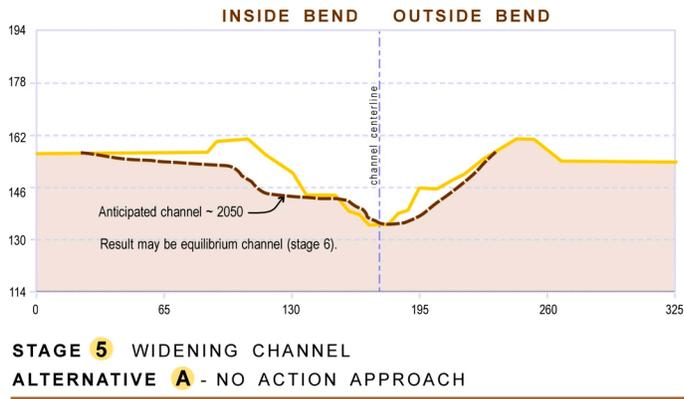
Figure 13. Typical existing conditions and conceptual design for Reach 3
