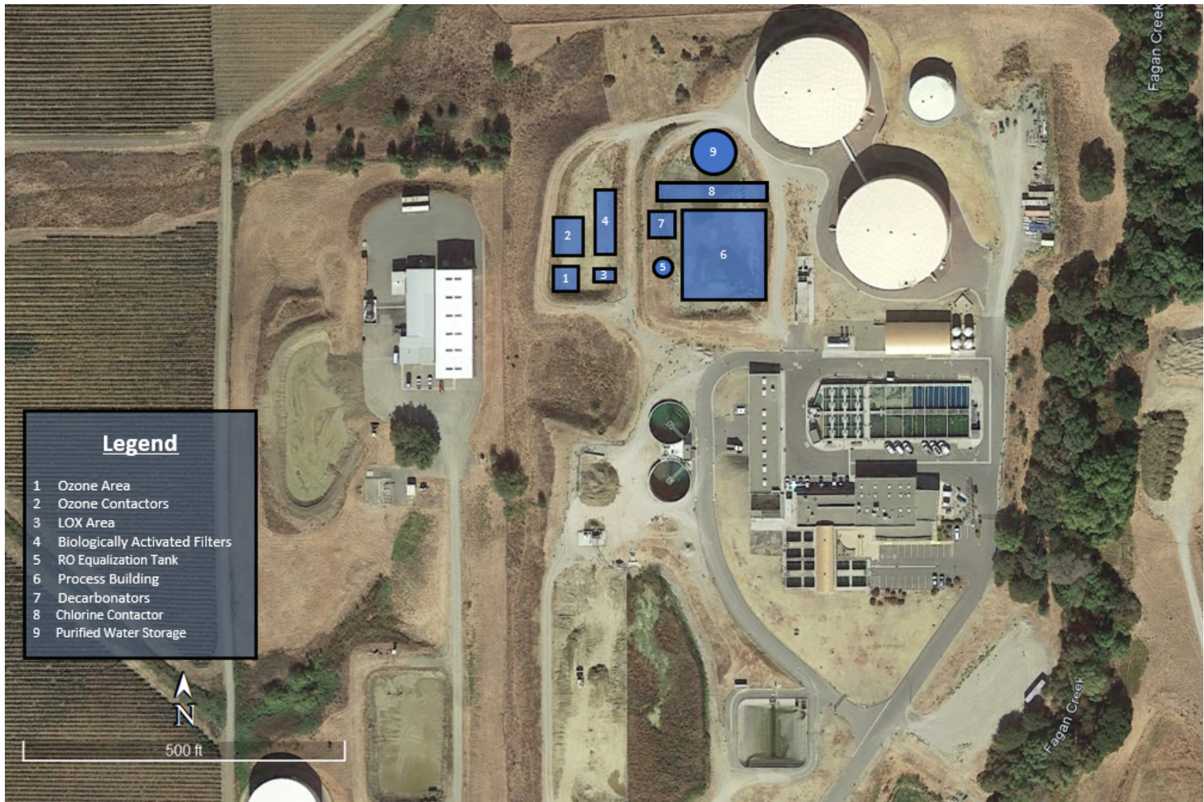
Figure 3-1. Site layout for RWA at the Jamieson WTP
