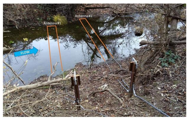
Figure 7. Paired PIT tag antenna loops in the Napa River.
