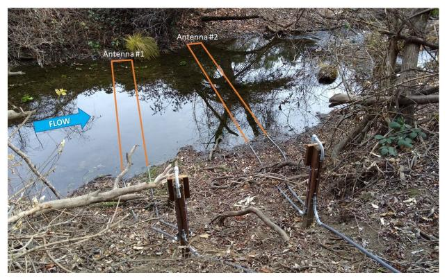
Figure 10. Paired PIT tag antenna loops in the Napa River.
