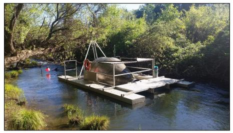
Figure 1. Napa River rotary screw trap
