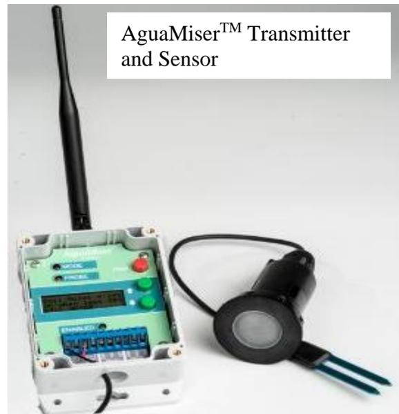
AguaMiser MZ (multi-zone) units can control and monitor up to 64 wireless transmitters and soil sensors, with web-based data collection and reporting.
