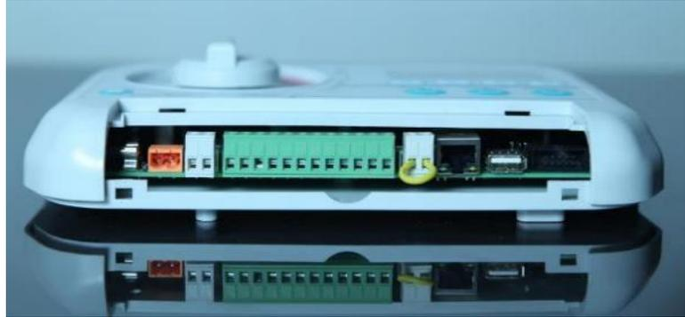
NxEco controllers are designed for indoor installation, but an optional outdoor enclosure or cabinet (UCC100) is available. The cabinet dimensions for the controllers are 6.5 by 9.8 by 1.4 inches.
