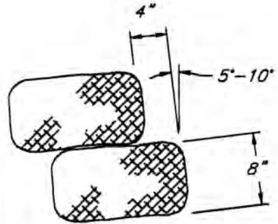
*Constructed with continuous berm machine (CBM) using 6-12oz./yd. non woven geotextile filter fabric filled with native soil, sand or gravel.*
