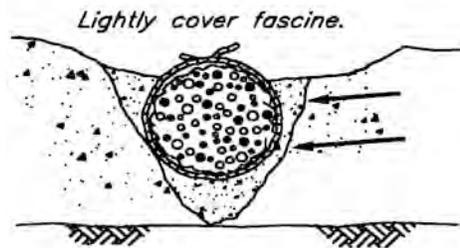
Place bundle of cuttings (fascine) in the trench and lightly backfill with native material.
