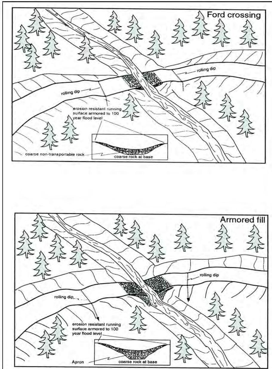
Figure X-15. Typical ford and armored fill stream crossings.
