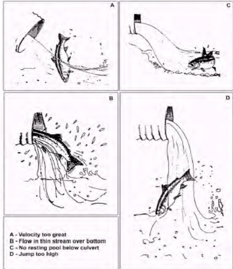
**Figure 4.2 Fish passage barrier conditions at culverted stream crossings.** (California Salmonid Stream Habitat Restoration Manual; Chapter IX, California Dept. of Fish and Wildlife, Flosi et. al 2002.)
