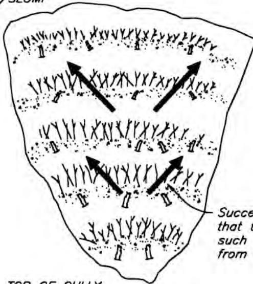
*Successful brushpacking requires that the gully be filled convex such that runoff drains away from the center.*
