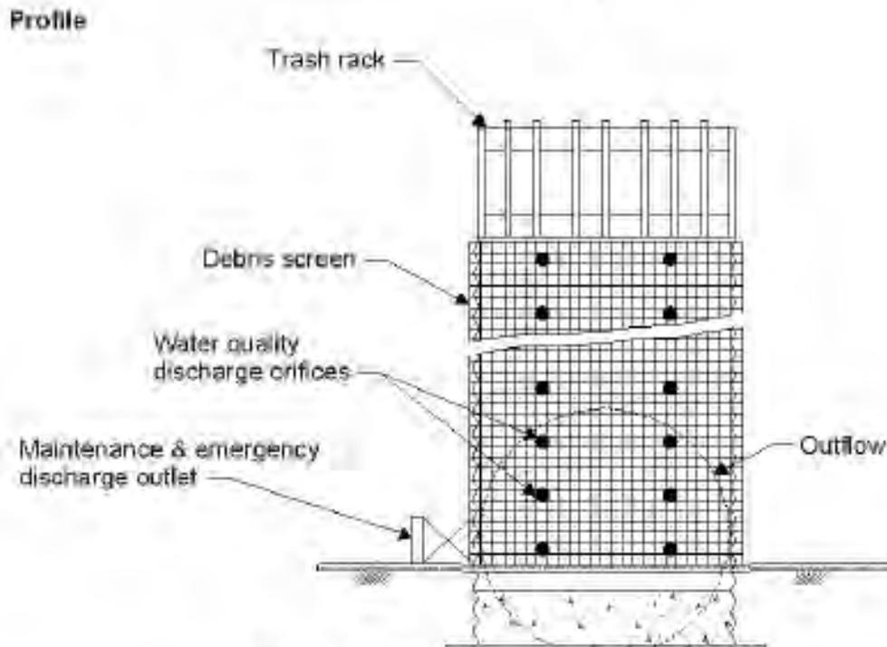
**FIGURE 3: MULTIPLE ORIFICE OUTLET RISER
