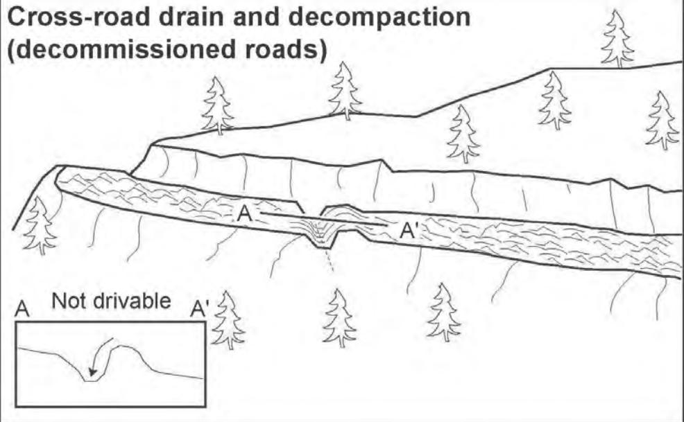
Cross road drain construction will ensure gullies, springs, road runoff and other concentrated flow will no longer collect over long lengths of road causing gully erosion and sediment delivery to streams. Cross road drains will be constructed at approximately 75 ft spacing intervals and these cross road drains will direct road surface runoff off the road onto stable hillslope locations.
