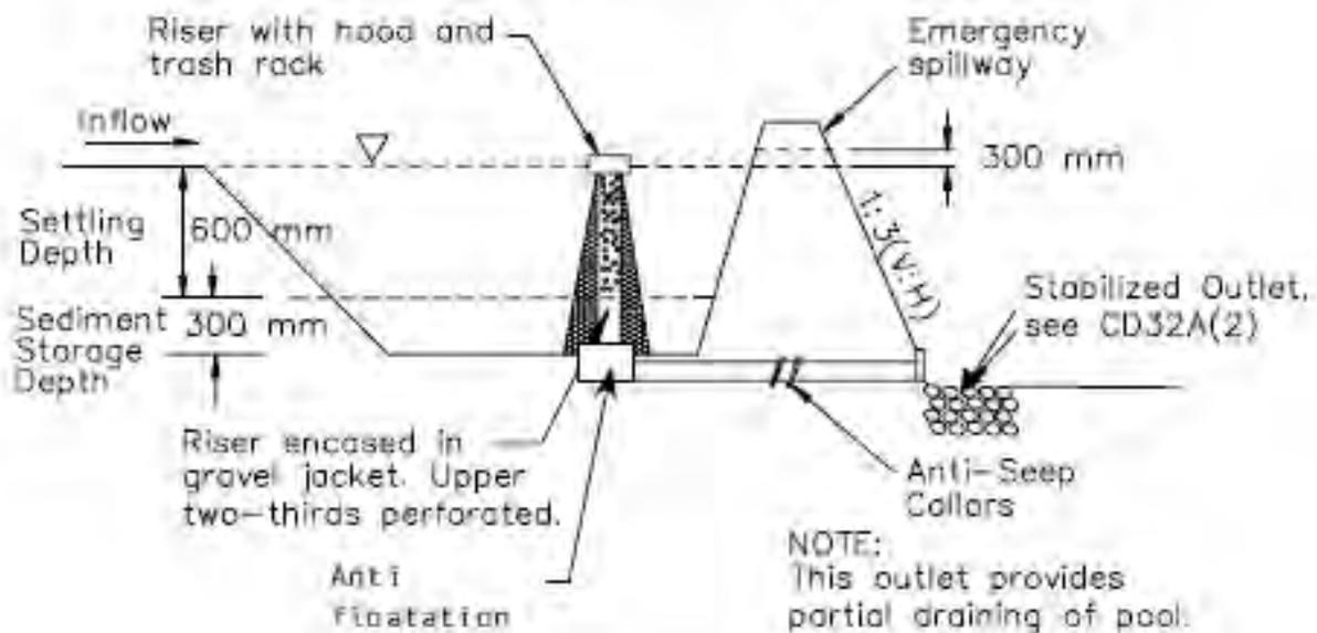
**FIGURE 2: MULTIPLE ORIFICE DESIGN**
