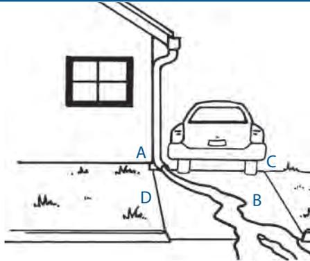
**B** This driveway slopes toward the street and creates runoff potentially contributing to flooding, erosion, and pollutants in nearby storm drains and streams.
