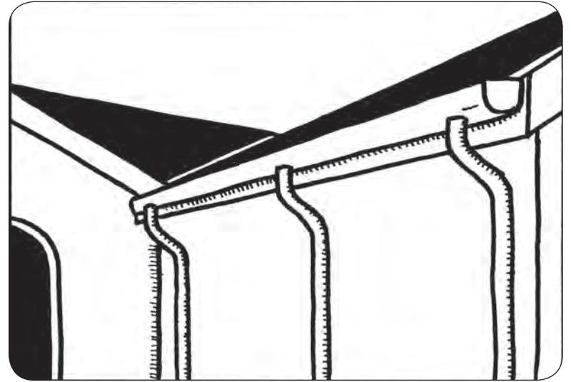
Adding an additional downspout helps reduce the volume and velocity of runoff at any given point thereby reducing the potential for erosion.
