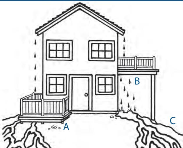
**A** Low decks may prohibit the addition of protective ground cover, leaving bare soil to erode.
