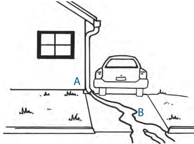
**A** The downspout is directed toward an impervious (concrete) driveway. Instead of infiltrating into the soil, the runoff will flow down the driveway and out to the street.
