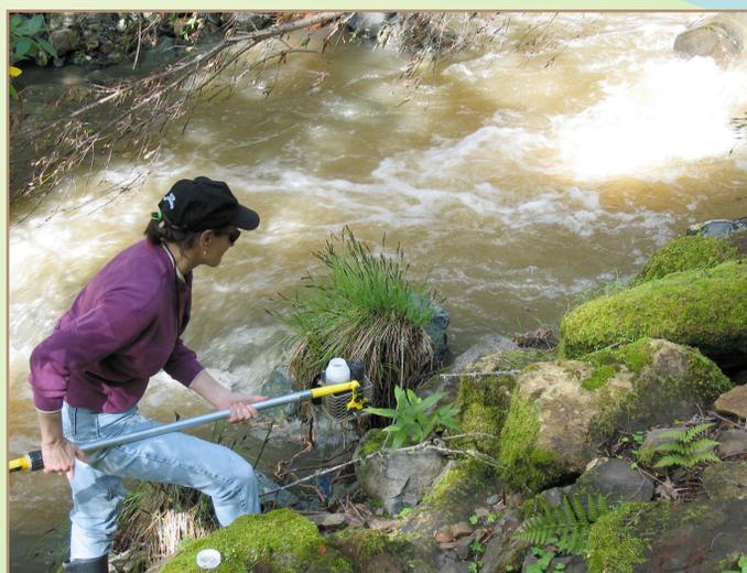
**2002 to present**—Suspended sediment monitoring is conducted at continuous automated station and grab-sampling locations, as empirical check on source estimates.
