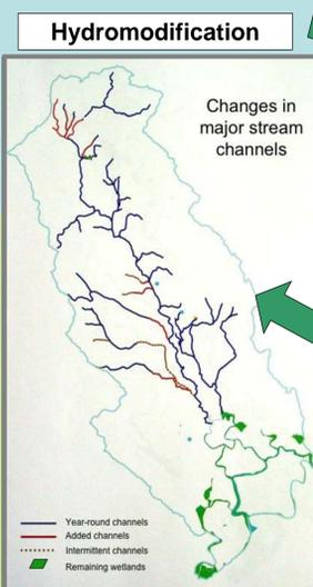
**Channel connections and straightening** were largely completed by 1877. Increased ditching, piping, and hardening of surfaces followed.
