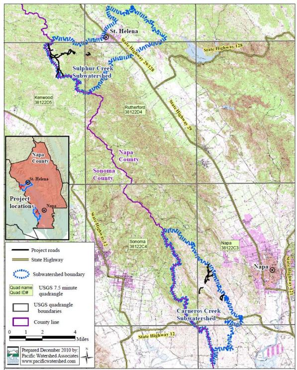
Map 1. Locations of project roads in the Cameros Creek and Sulphur Creek subwatersheds. Demonstrating Road Improvements in the Napa River Basin: Implemented Road Treatments to Reduce Erosion in the Cameros Creek and Sulphur Creek Subwatersheds, Napa County, California.
