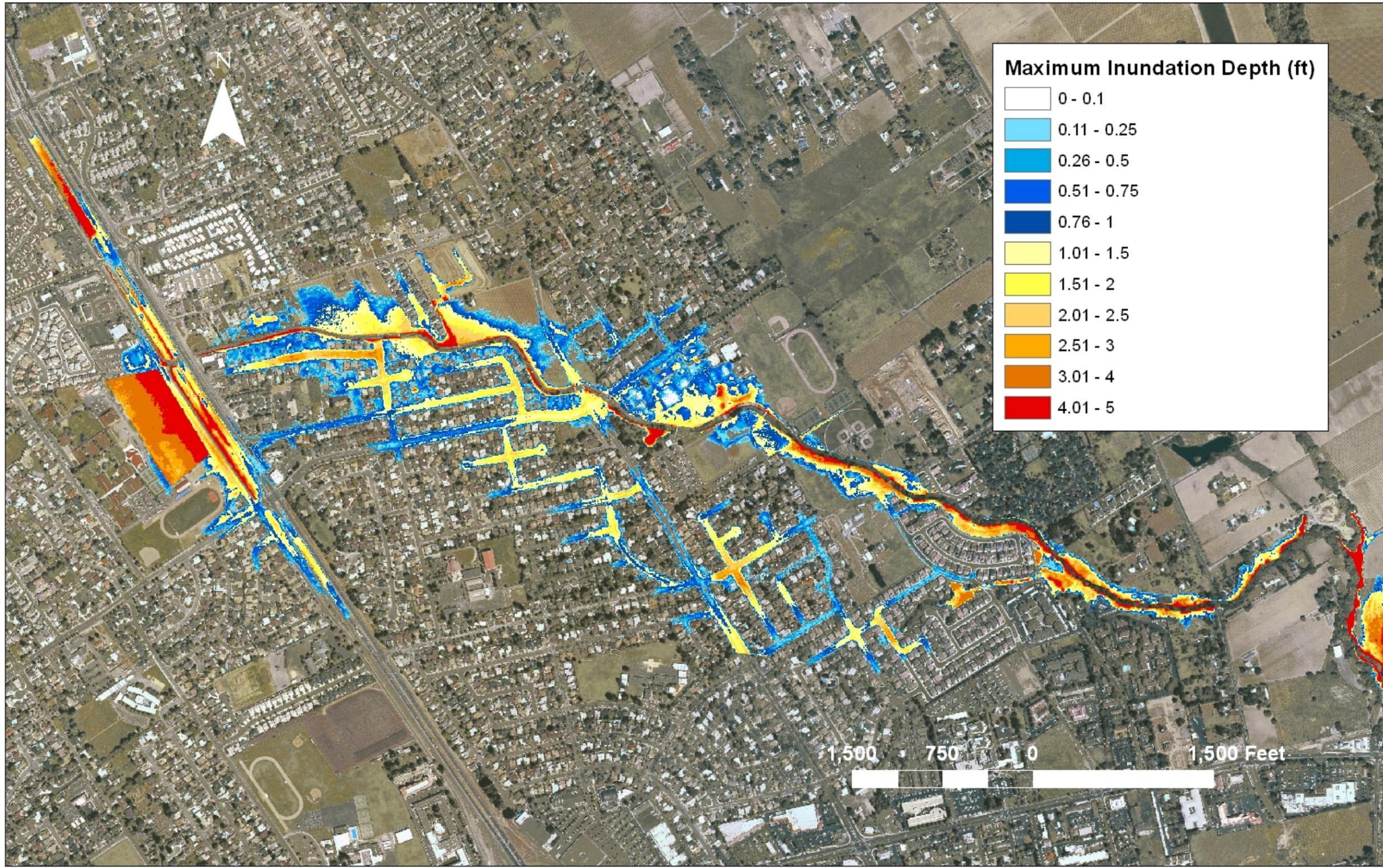
Figure 20. Maximum inundation depths (ft) for the 100-year flood event for Scenario 4
