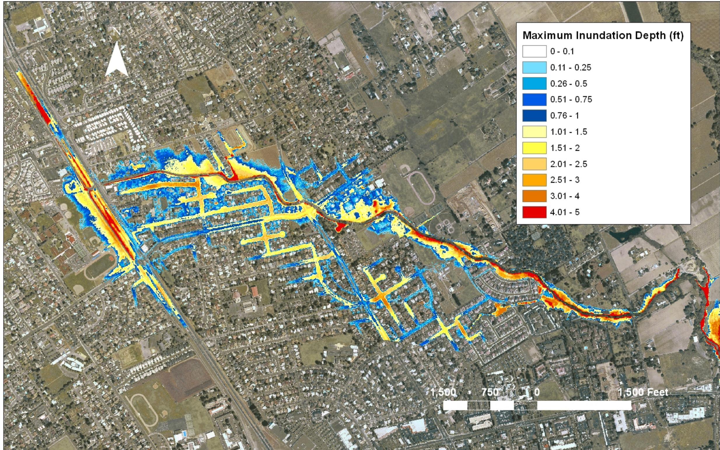
Figure 7. Maximum inundation depths (ft) for the 100-yr flood event
