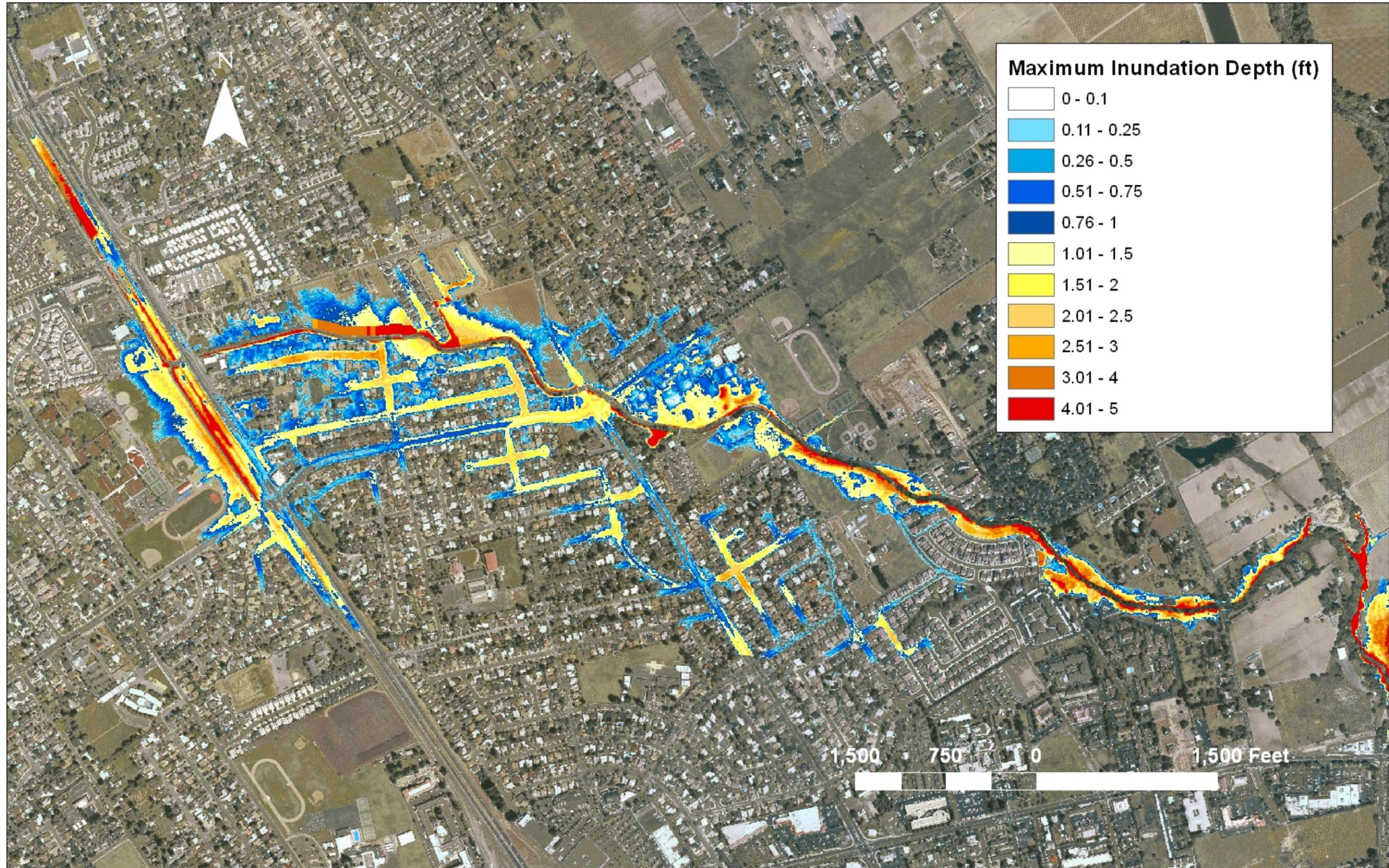
Figure 15. Maximum inundation depths (ft) for the 100-year flood event for Scenario 3
