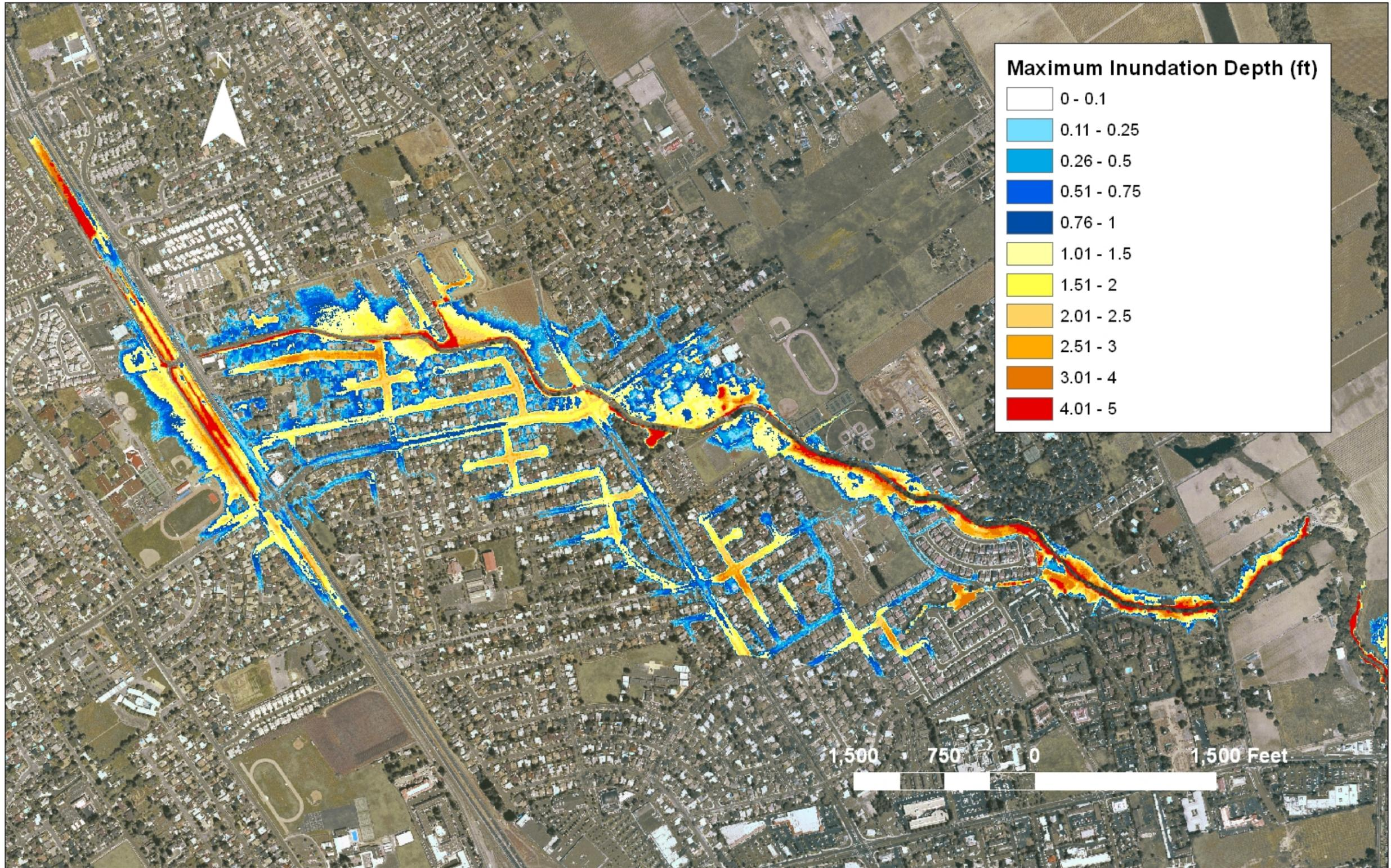
Figure 13. Maximum inundation depths (ft) for the 100-year flood event for Scenario 2
