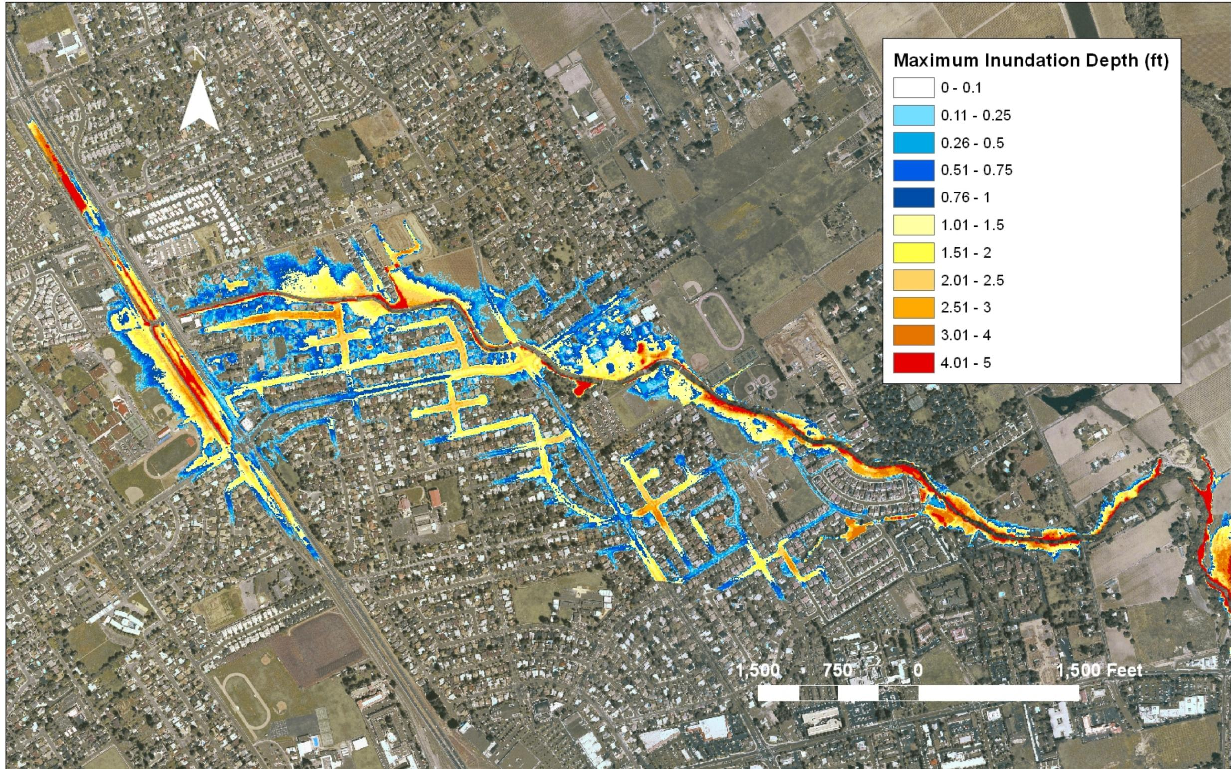
Figure 10. Maximum inundation depths (ft) for the 100-year flood event for Scenario 1
