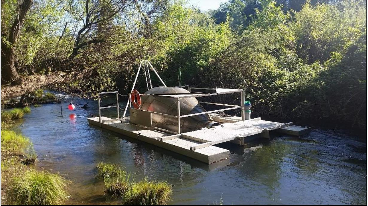
Figure 1. Napa River rotary screw trap
