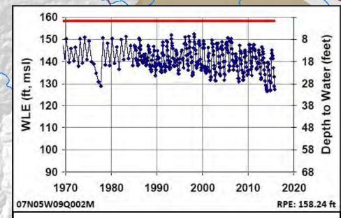
Well 07N05W09Q2 is constructed in an area where alluvial sediments extend to approximately 200 feet below ground surface (LSCE and MBK, 2013). Static groundwater levels in this well typically vary by about 20 ft from spring to fall and have remained well above the bottom of alluvium, indicating significant contributions from the alluvial aquifer system.
