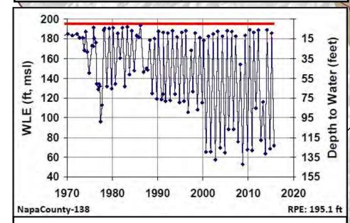
Well NapaCounty-138 has a total depth of 321 ft and is located in nearer to the Napa Valley margin in an area where alluvial sediments extend only approximately 50 feet below ground surface (LSCE and MBK, 2013). Static groundwater levels in this well indicate increasing contributions from geologic formations below the alluvium, although spring season groundwater levels have remained stable.
